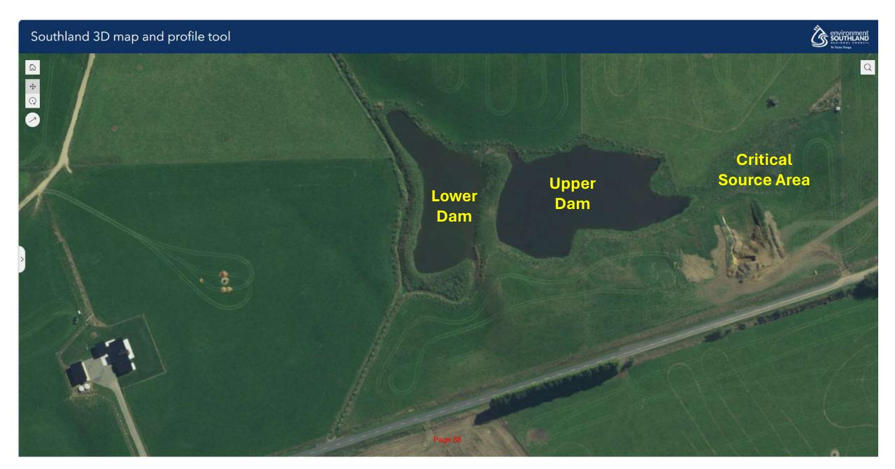
Looking South (downstream) from the head of the wetland complex which consists of three distinct components – a lower dam, an upper dam, and a fenced-off critical source area (with some native planting) upstream of the upper dam.
