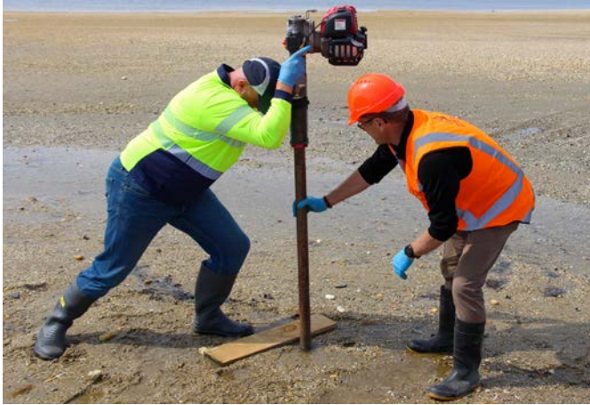
▲ Environment Southland Tiwai technical lead Graeme McKenzie (right), assists EHS Support's smelter expert Warren Sharp, with a demonstration of core sediment sampling for the independent coastal monitoring programme to address gaps in data on the environmental impacts of the Tiwai smelter.
