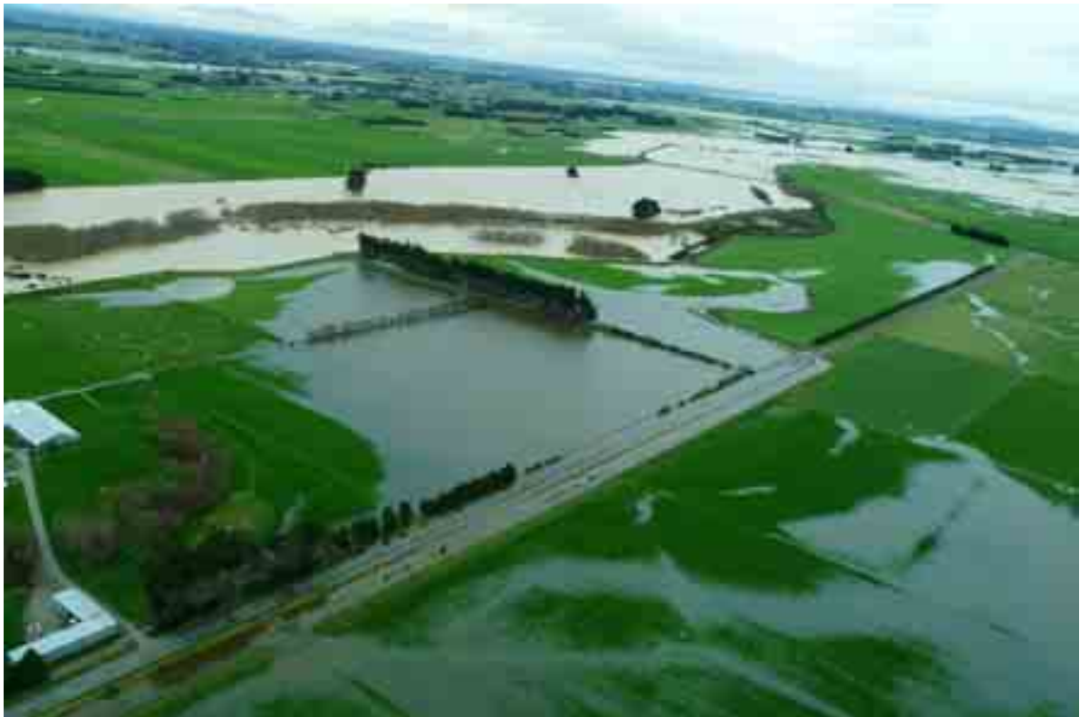
Southland's extensive rural stopbanking systems are designed to protect from medium size floods and give farmers time to reduce the effects of large floods [Dave Connor]
