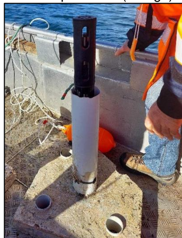
Figure 2: Turbidity logger deployment set-up.
