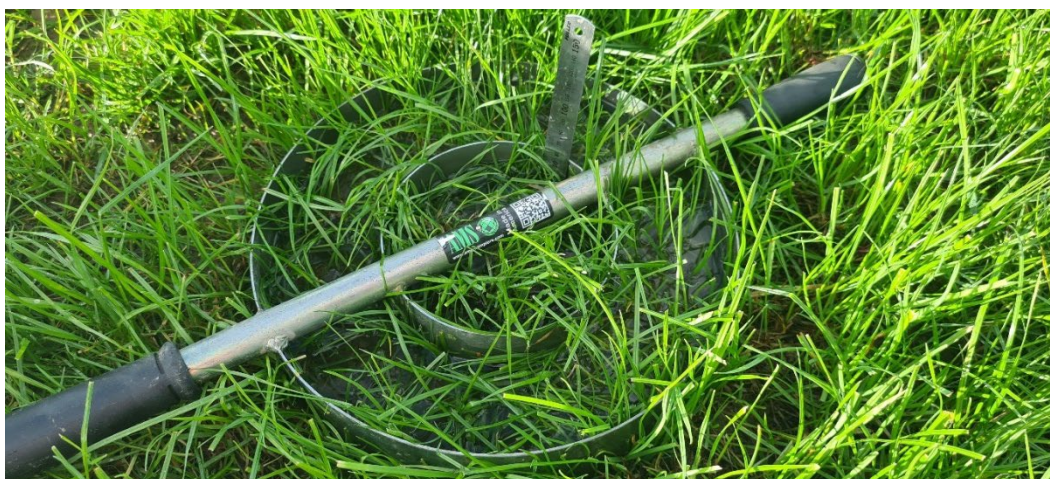
Figure 10: Double ring infiltration setup for soil infiltration testing. During use, both rings are filled up with water with only the inner ring measured. The reason for only measuring the inner ring is the outer ring may infiltrate much faster than the inner ring because there will be lateral movement of water around the cutter blade. This action also creates a seal for the inner ring and gives a much more accurate indication of the actual rate of infiltration at the location.
