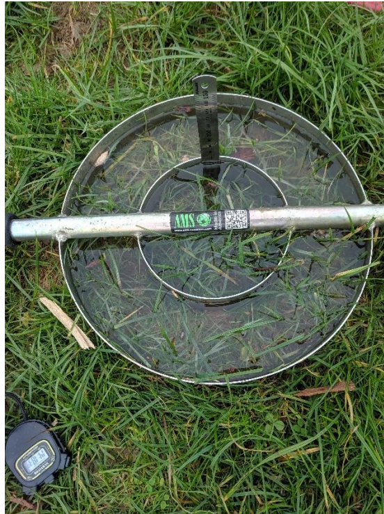
Figure 10: Double ring infiltration setup for soil infiltration testing. During use, both rings are filled up with water with only the inner ring measured. The reason for only measuring the inner ring is the outer ring may infiltrate much faster than the inner ring because there will be lateral movement of water around the cutter blade. This action also creates a seal for the inner ring and gives a much more accurate indication of the actual rate of infiltration at the location.
