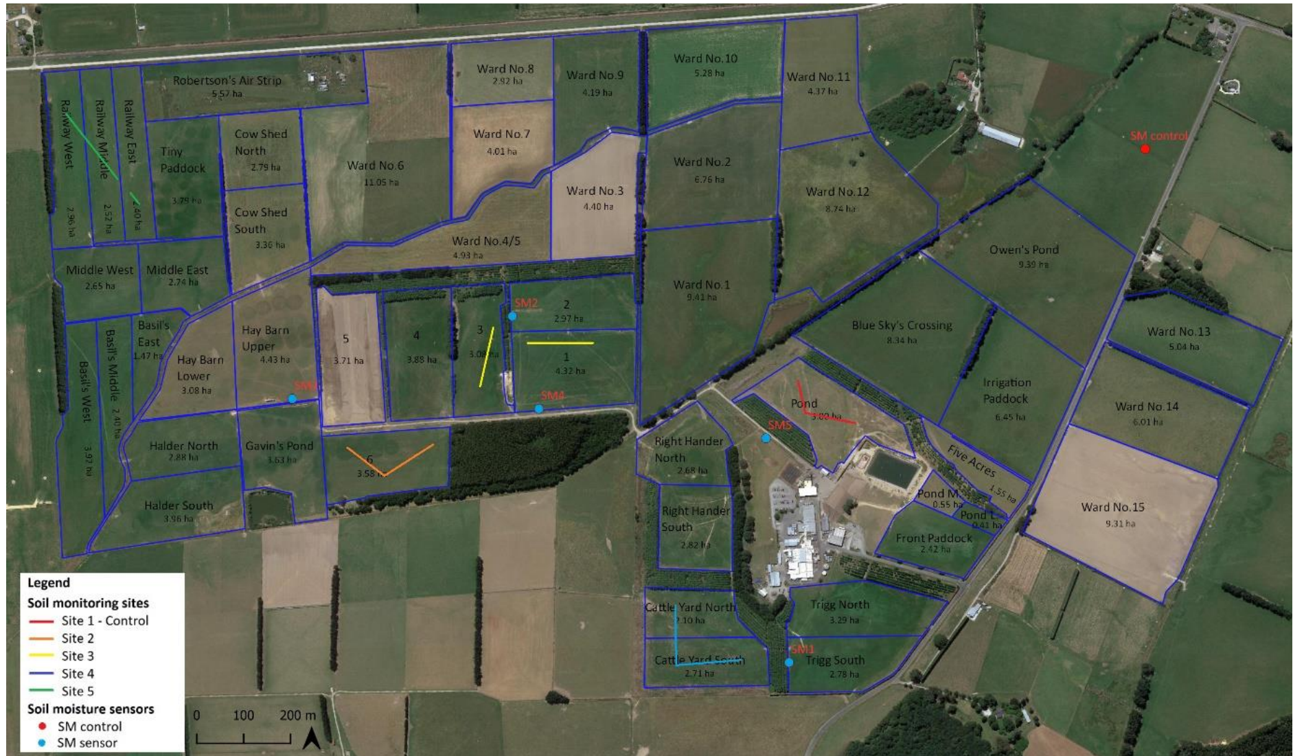
Figure 1: Soil sampling sites at Blue Sky Pastures, Morton Mains Plant. Coloured transect lines show where soil samples were taken at the monitoring sites. Where SM Control and SM1 – 5 denote the location of in situ soil moisture (SM) instruments used for irrigation scheduling. Note: Aerial photography is older than the second pond construction.
