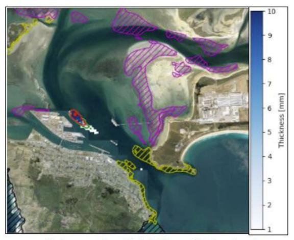
Worst-case sediment footprint (from a P3 release location over a spring tide cycle from 1 h before to 4 h after high water) with seabed resuspension excluded. The green and red contours highlight 2 and 4 mm respectively. The purple, yellow and black hatched patch represents the seagrass, rocky and mataitai area respectively. Deposition thickness of less than 1mm were masked (from Zyngfogel & McComb, 2023).
