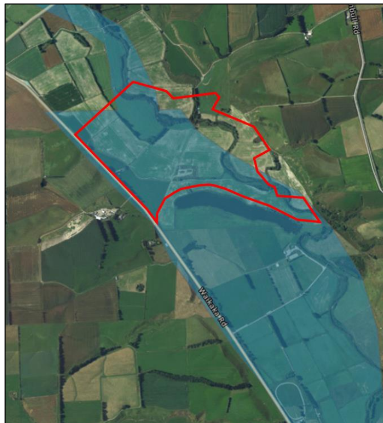
Figure 30 Area subject to inundation indicated in blue. Site extent indicated in red outline
