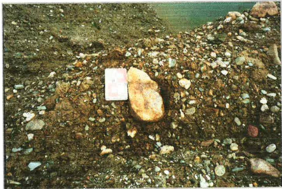
Figure 8. The river flows through old dredge spoil which is composed of gravels and some boulders contained in a silt/clay matrix. (The notebook is 185 by 115 mm).
