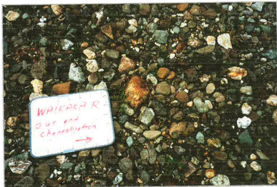
Figure 10. Bar surface materials in the undisturbed reach are relatively coarse ( D_{50} \sim 20 mm). This armour layer overlays much finer material. (The grid lines on board are 50 mm).
