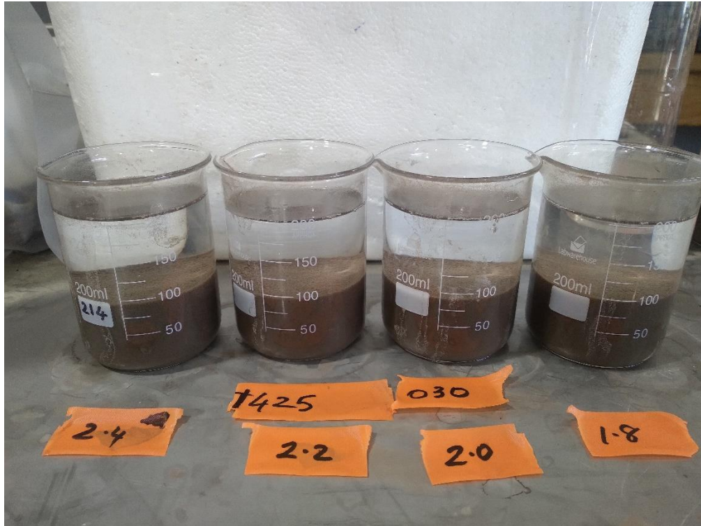
Figure 6: Sample 30. 1.8, 2.0, 2.2 and 2.4 ml of 1% solution of Magnafloc 1425 mixed with diluted dirty water
