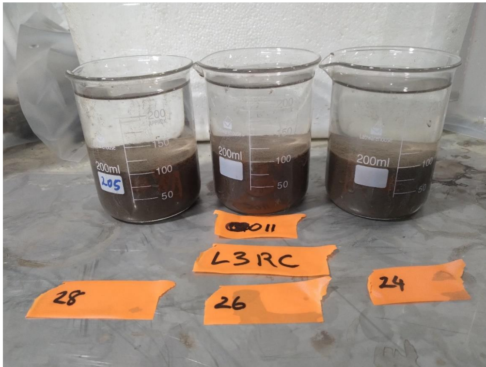
Figure 2: Sample 11. Photograph after 15 minutes of samples where 24, 26 and 28ml of 0.001% solution of Crystalfloc L3RC was added. Clear supernatant.
