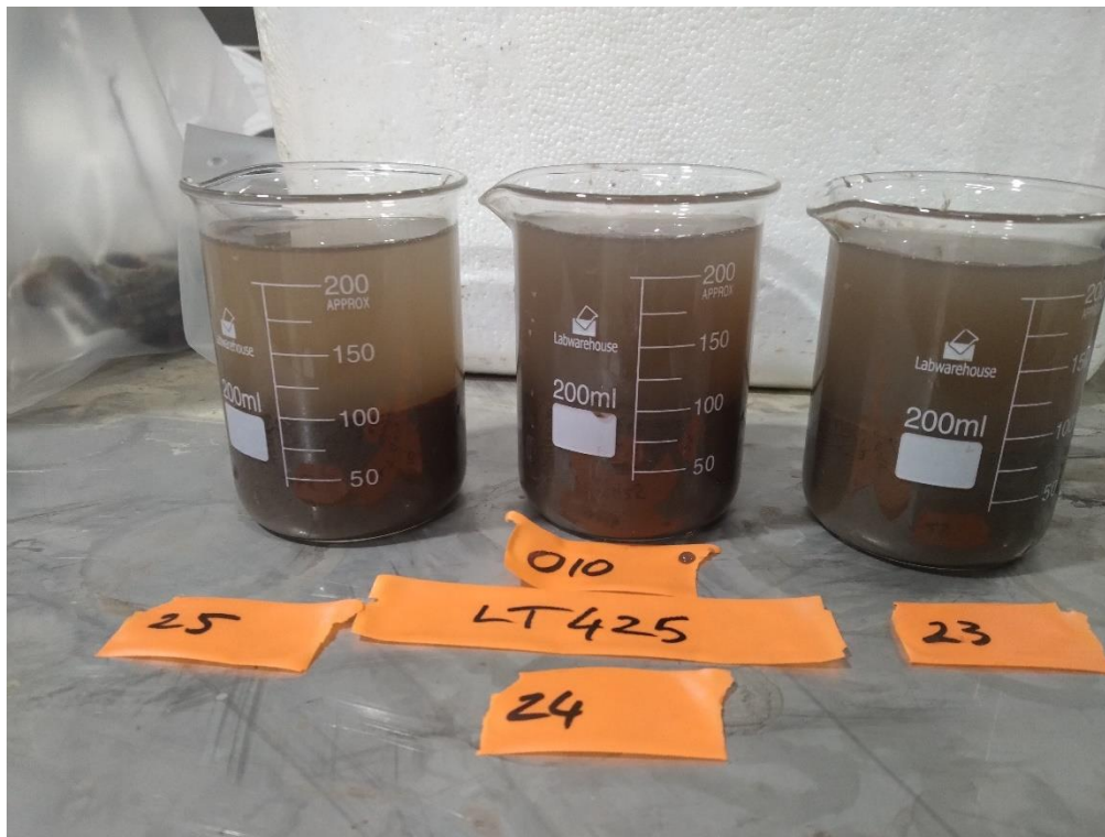
Figure 1: Sample 10, after addition of 23, 24, and 25ml of .001% solution of Magnafloc 1425 to each 200ml sample of dirty water. Note that supernatant is still quite dirty.
