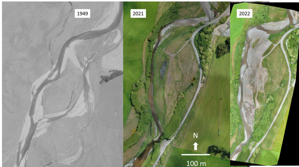
Figure 12. Whitestone River at McGregors, 1949 (original, natural condition), 2021 (pre-skimming), 2022 (post skimming). Source: Retrolens and ES. Flow is from north to south, scale approximate.
