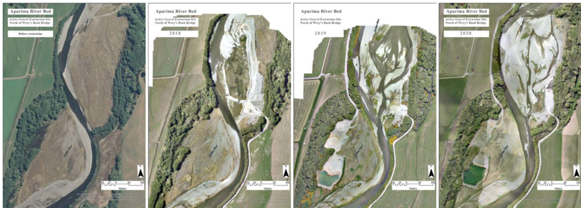
Figure 11. Sequence of aerial images showing Aparima reach at Wrey's Bush pre-treatment (left), mid-treatment in 2018 and post-treatment in 2019 and 2020. Note: flow is from north to south. Removal of the thick sward of grass and soil developed in the active channel has returned the channel to a form resembling its condition in the 1950s (cf. Figure 9). This also displays a contrast between traditional approaches to gravel extraction, which stay away from the water, restrict surface disturbance, dig deep holes, which leave ponds, visible in the adjacent downstream bar. Source: Lagrue & McGregor Aparima River Restoration Project, DoC presentation, 8 June 2021.
