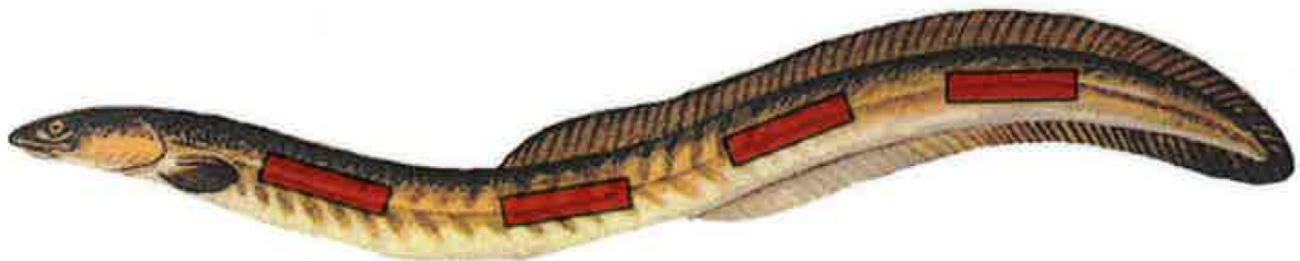
Figure 2: Four fat meter readings were taken along each side of the eels (8 measurements total). Image taken from Distell calibration card, “EEL-2”
