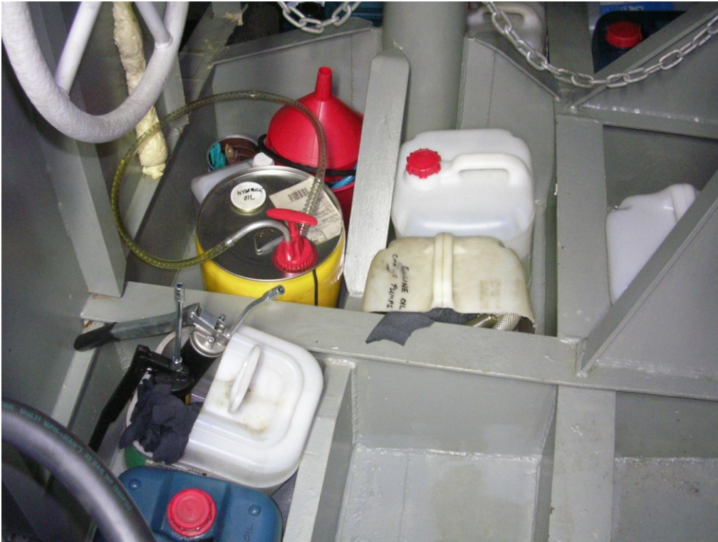
Figure 2: Bunded compartments for storage of hazardous chemicals etc.
