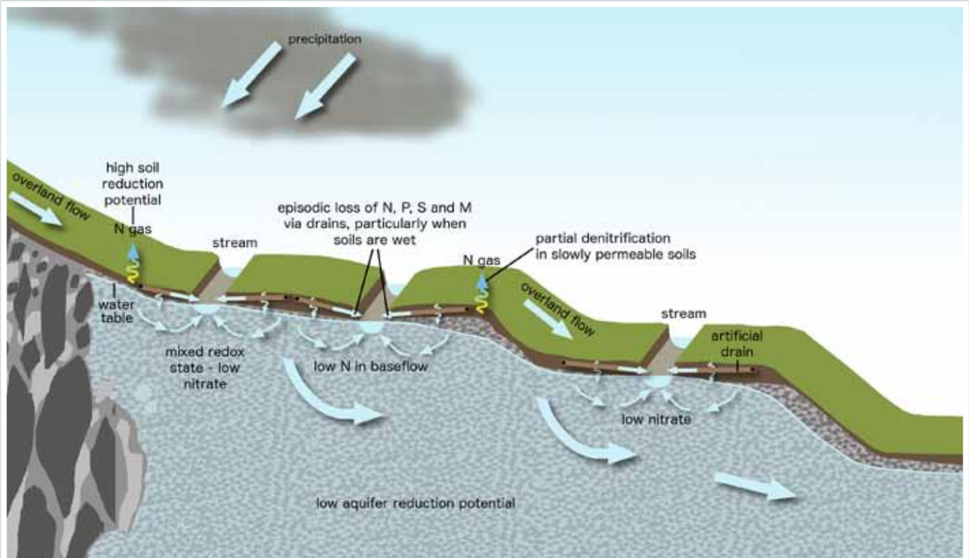
▲ Figure 2: Main zone – Deep drainage to groundwater typically contains low nitrate concentrations due to denitrification within poorly drained soils.
