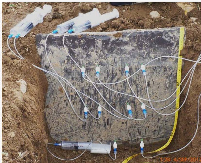
Figure 4-5: Example of Teflon suction cup deployment in a Southland soil. The steel plate is hammered into the soil and an awl (a narrow diameter spike) of slightly smaller diameter than the suction cup is made through drill holes within the plate. A paste of soil and deionised water is used to seal the cups and suction is applied and left for 18 – 24 hours before collection.
