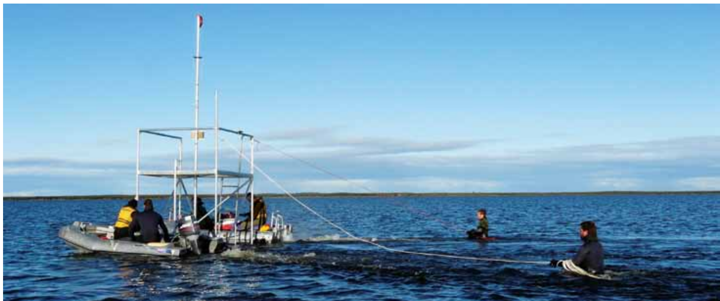
The monitoring platform was towed out into the lagoon before being anchored into place. The platform will provide real-time data about water quality and weather conditions.
