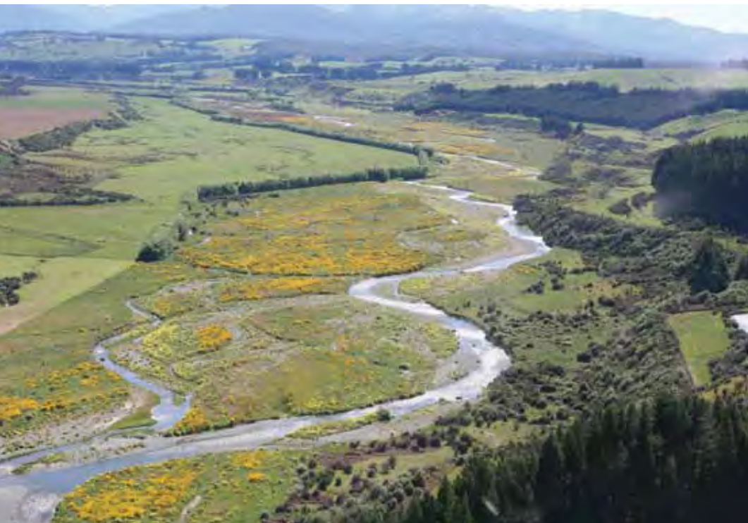
An aerial survey of the Upukerora River shows areas which need to be sprayed to keep the floodway clear to ensure flood flows can pass.
