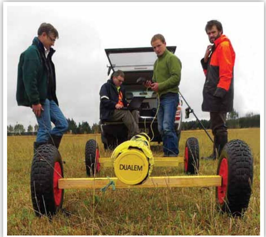
The new conductivity meter enables scientists to take a look beneath the surface.
