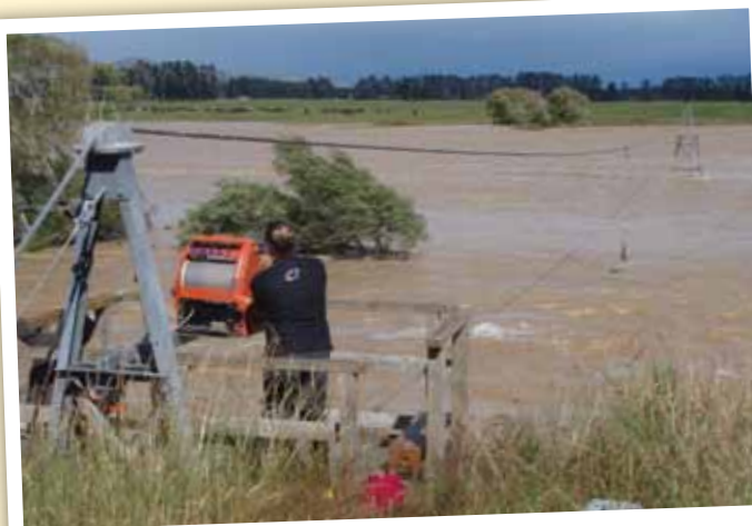
During the January floods, Environmental Data staff were out measuring river depth and flow velocity on the Oreti River. They had to watch out for trees travelling down the raging torrents, threatening to catch in the cable carrying the measurement device known as a 'poem'.
