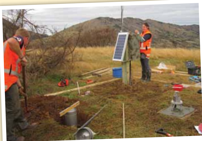
One of Environment Southland's roles is providing flood warning for the Southland region. Staff from the Environmental Data team installed a new rain gauge along the upper Oreti River to measure the rainfall that feeds the river and contributes to floods. With plenty of rock breaking it was very hard to dig holes to install the equipment.
