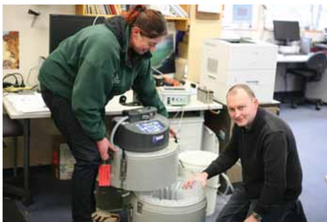
Water Auto Sampler – Senior hydrologist Chris Jenkins and senior environmental technical officer Stacey Stuart take a look at one of six new auto samplers about to be installed. The auto samplers are pre-programmed to take samples from rivers and will be particularly useful during periods of high rainfall.
