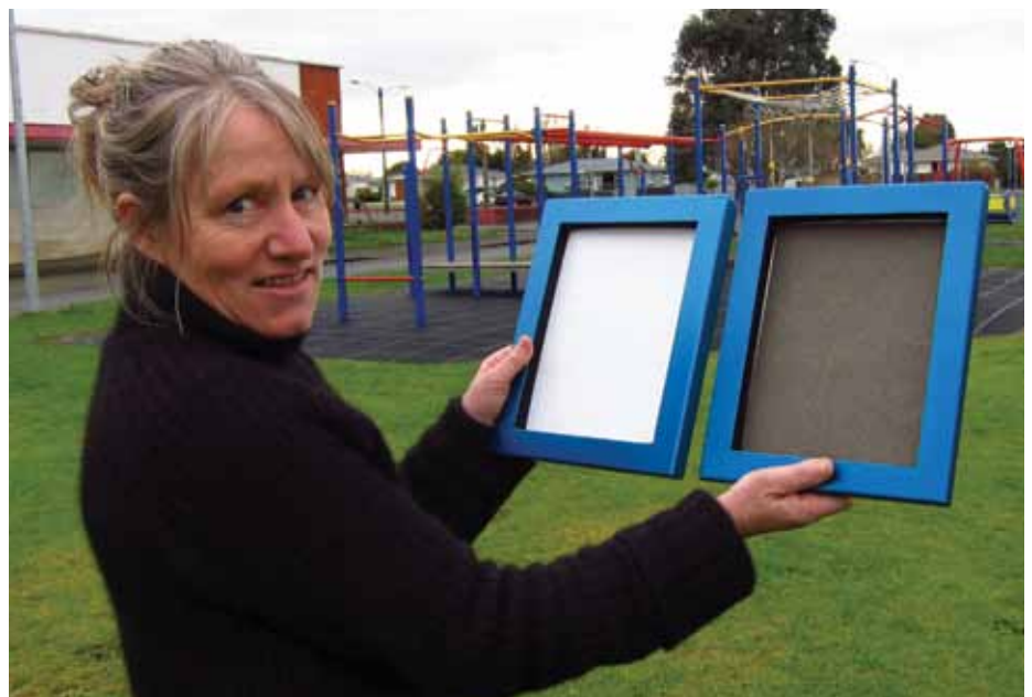
Environment Southland technical officer, Wendy Barrow, with a new air filter (left) for a high volume sampler and a used filter turned black from PM 10 .
