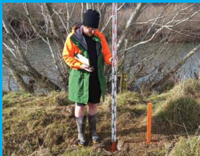
▲ Hydrologist Phil McCartney checks the correct height of a water level gauge in the Mataura River. The gauges are checked to ensure water level data is accurately recorded by our monitoring equipment.
