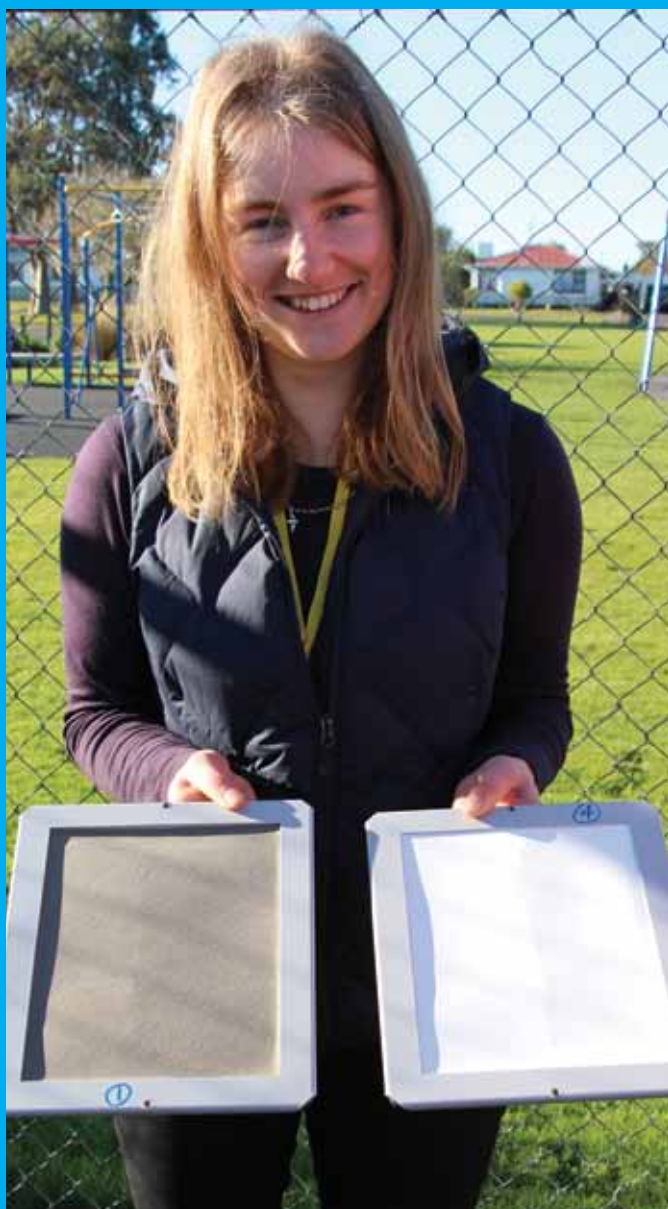
▲ Environmental technical officer Grace Smith changes air filters at the Glengarry monitoring station in Invercargill. The used dark filter on the left indicates heavy traces of PM_{10} , most of which is caused by emissions from home heating. The other is a clean replacement filter. Filters are changed every second day throughout the winter monitoring period from April to the end of August and then every six days during the rest of the year.
