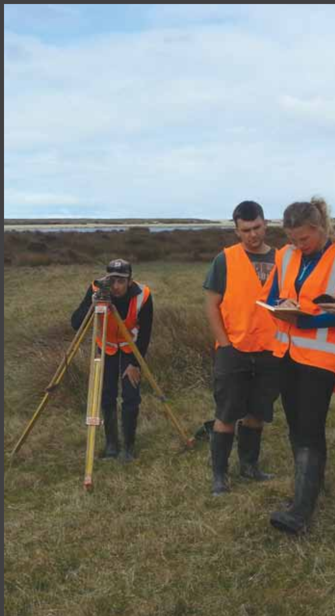
▲ Environmental technical officer Michael McDonald checks the level of a water height gauge at Waituna following maintenance adjustments, while Nathan Hughes and Lucy Just record measurements.
