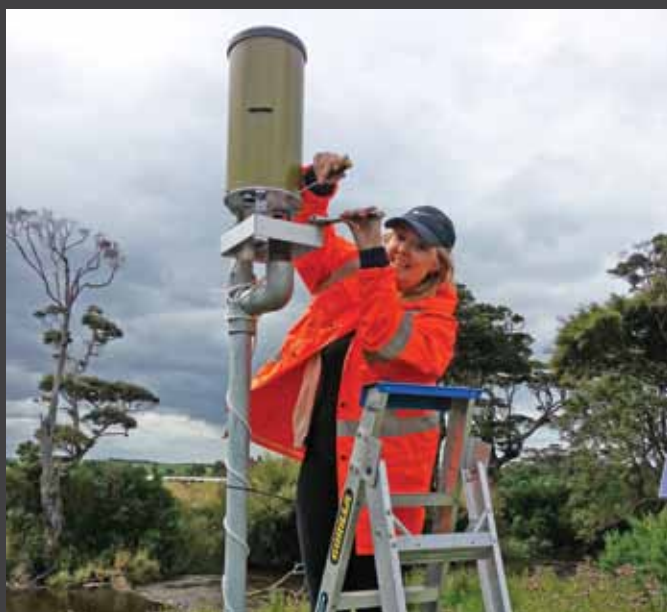
▲ Summer student Lauren Visser inspects a rain gauge on the banks of the Pourakino River. Live data from our rainfall monitoring sites is available on our website, and helps us monitor our water resources and forecast the likely size of a flood.
