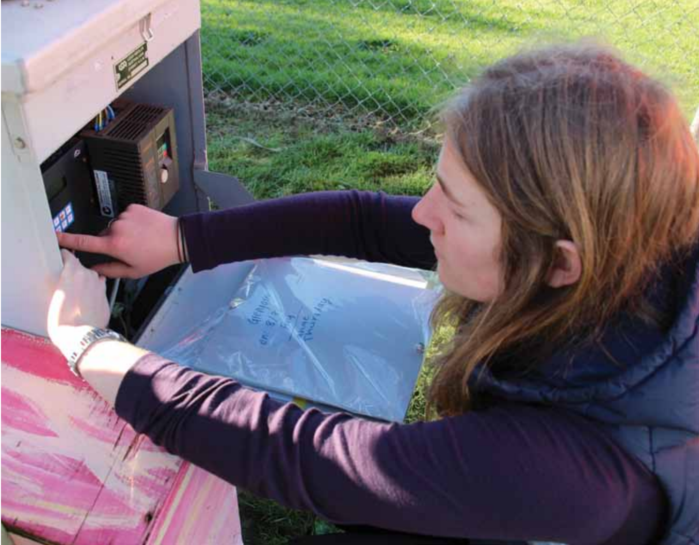
▲ Grace Smith checks air quality monitoring data and changes filters at the Glengarry monitoring station in Invercargill.
