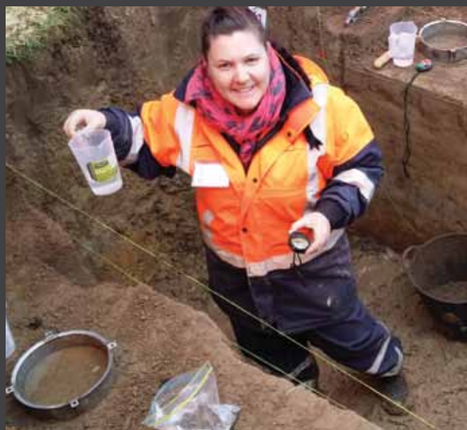
▲ Soils and water scientist Lisa Pearson measures soil infiltration rates in a Woodlands soil pit. This helps provide information on how different soils are able to absorb rainfall or irrigation.
