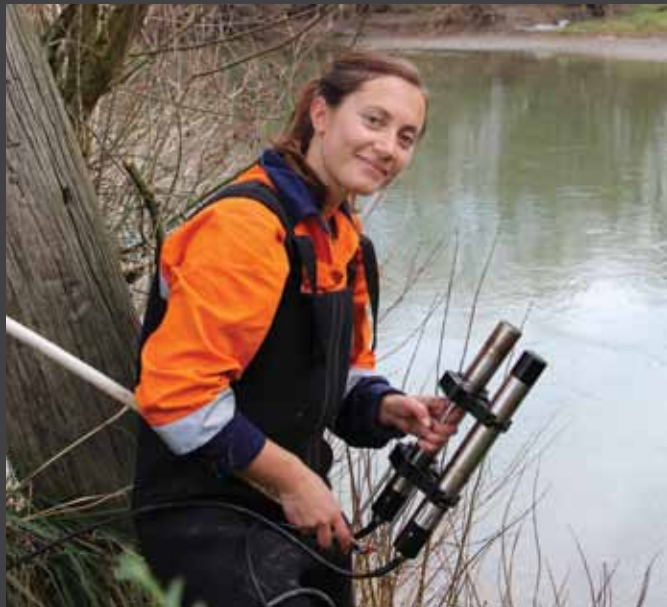
▲ Environmental technical officer Alice Woodward checks turbidity and conductivity probes in the Oreti River. The probes operate continuously and provide valuable water quality information throughout the year.
