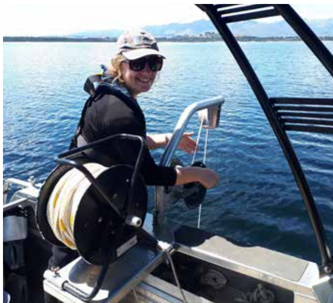
▲ Senior environmental technical officer Grace Finlayson uses a secchi dish to measure visual clarity on Lake Manapouri.
