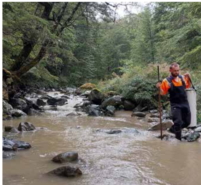
▲ Science assistant Jeremy Littlejohn collects deposited fine sediment samples with a quorer at McKay Creek on Milford Road.
