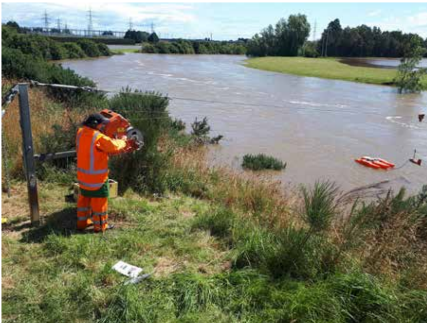
▲ Environmental technical officer Tessa Scully carries out high-flow gauging at the Makarewa River at Counsell Road monitoring site during the February 2020 flood.
