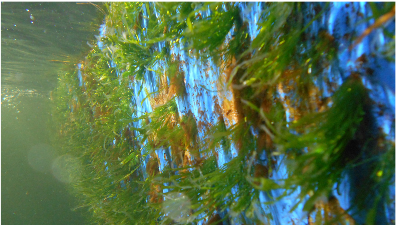
▼ Vessel with a fouled hull (DEREK RICHARDS, ENVIRONMENT SOUTHLAND)
