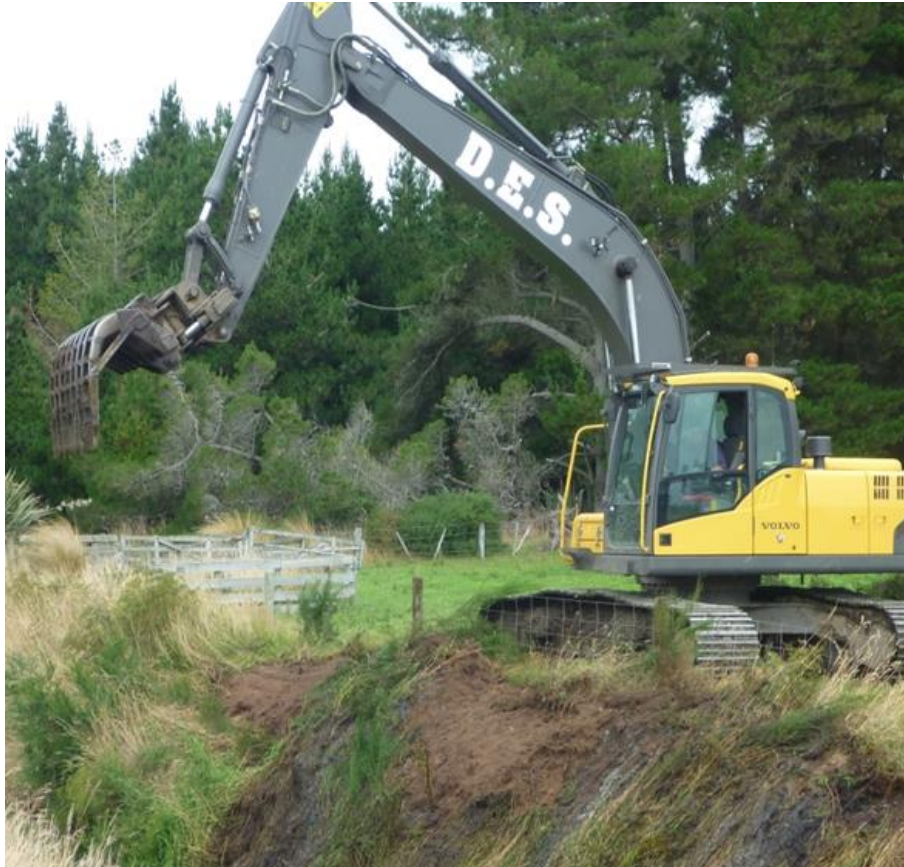
Figure 2: An example of a weed rake: Fish are able to swim through the large gaps and are less likely to be caught than if a standard bucket was used.
