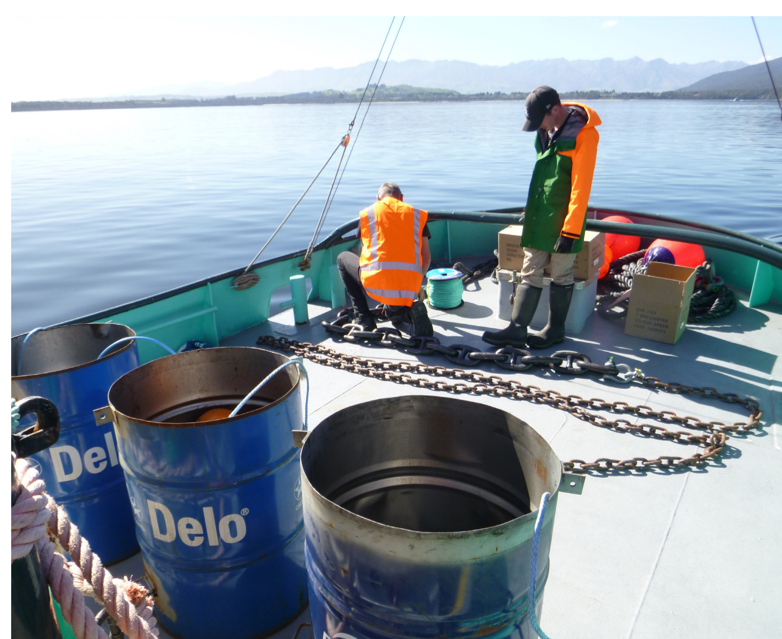
Figure 4: Deployment of one of the mooring arms.
