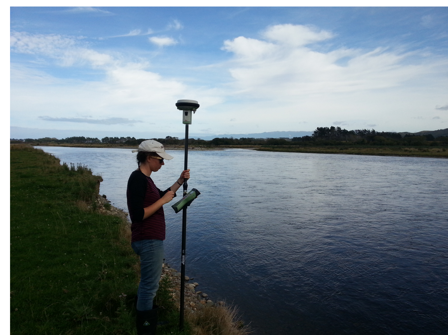
▶ A RTK measures bank erosion on the lower Waiau River site.
