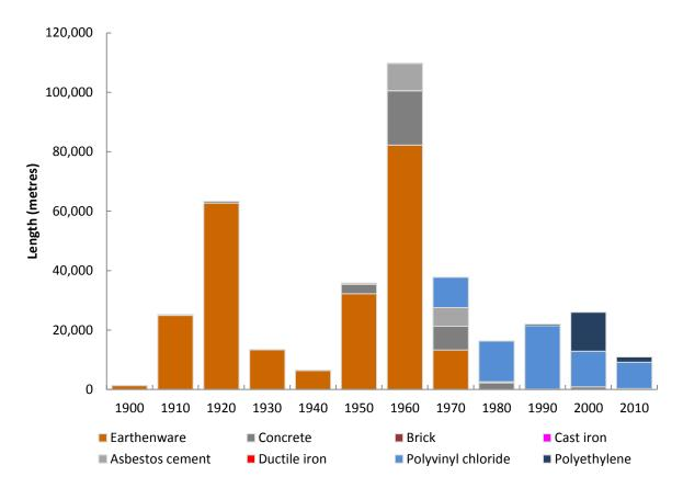
Figure 2: Invercargill wastewater reticulation
