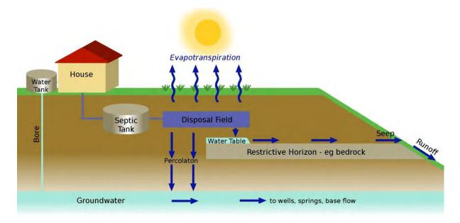
Figure 3: Flows of wastewater to and from a disposal field Source Ministry for the Environment
