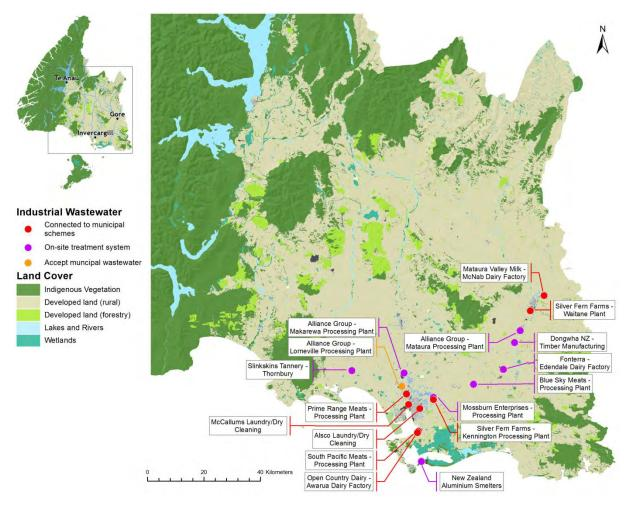
Figure B8: Location of key industrial wastewater discharges in Southland Source Environment Southland
