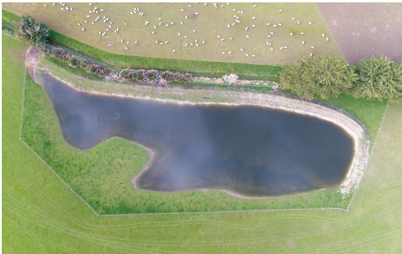
Constructed wetland treating field tile water before discharge into waterway
