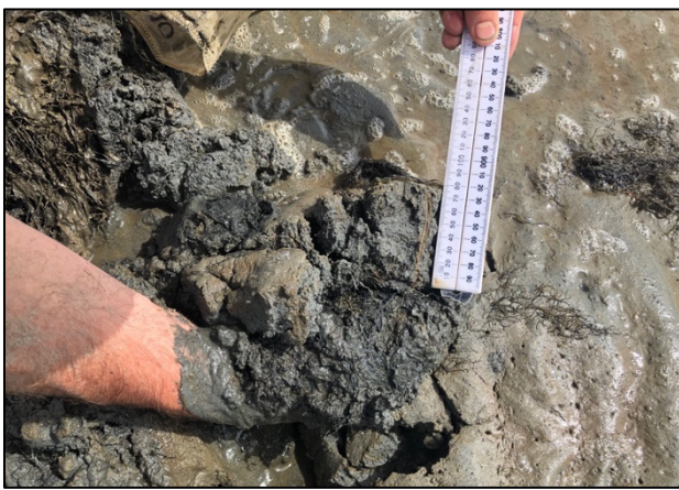
A 70mm layer of sediment relatively recently deposited on top of Gracilaria near Titiroa Stream
