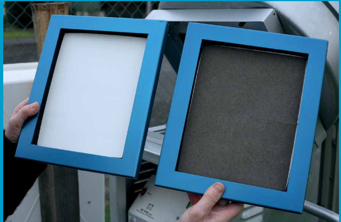
Figure 17: A fresh air filter (white) is compared with one that had been in use for two days during the winter of 2012 at the Glengarry Crescent air monitoring site in Invercargill.
