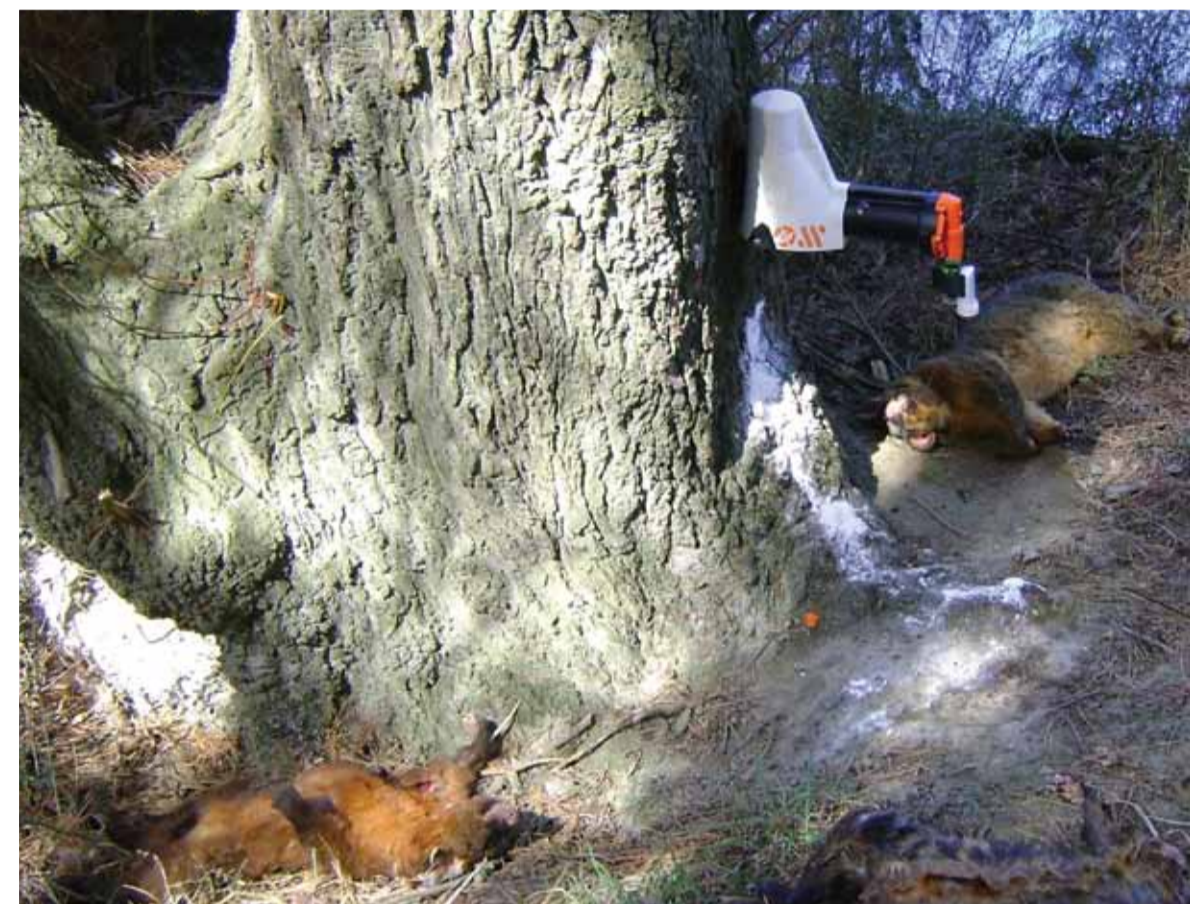
Goodnature automatic resetting kill trap
