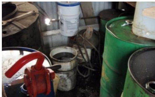
Figure 28 - Oil containers stored inappropriately
