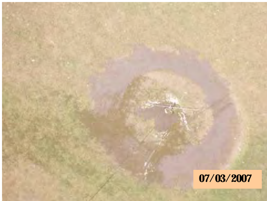
Figure 15 – Over-application of dairy effluent from a stalled irrigator discovered during helicopter inspections
