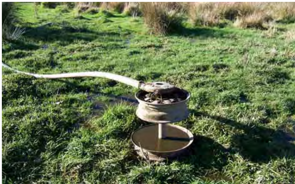
Figure 31 – Pot sprayer discharging truckwash waste
