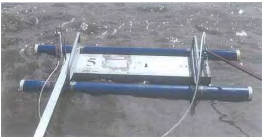
Figure 42 – The wind tunnel used to collect the surface odour emissions
