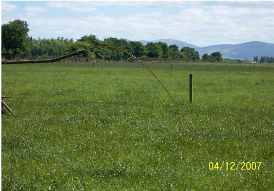
Figure 55 - Picture showing a travelling irrigator stalled and siphoning onto pasture.
