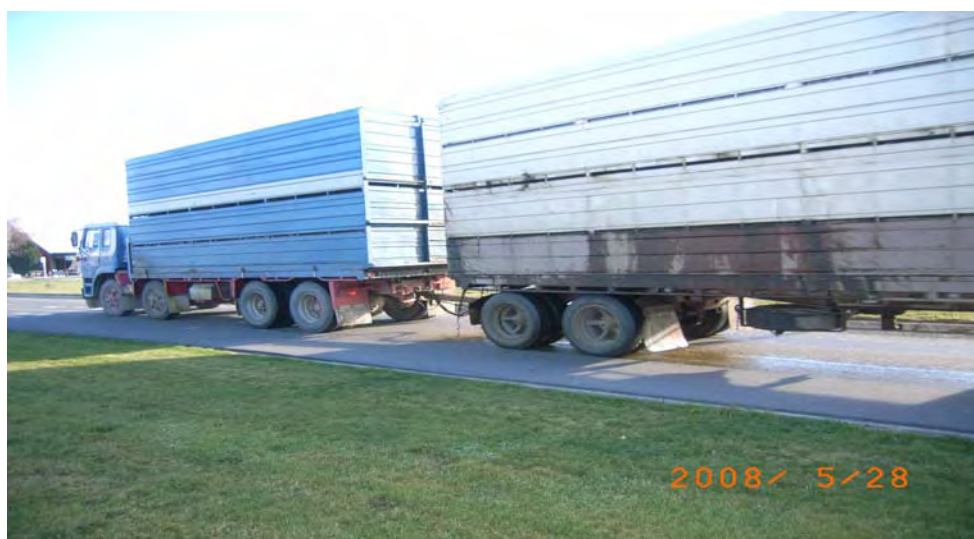
Figure 7 - Effluent leaking from a stock truck
