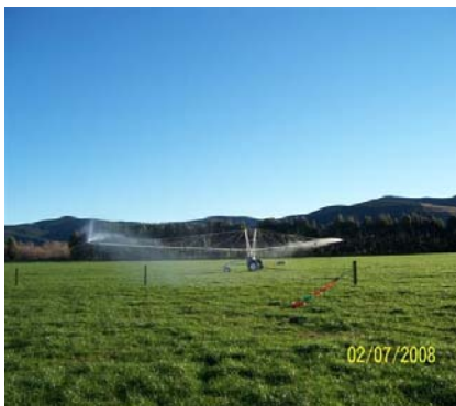
Figure 10 – Rotary boom travelling irrigator
