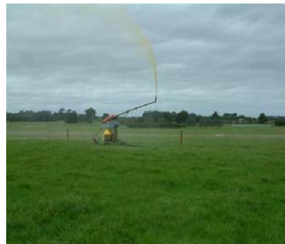
Figure 11 – Oscillating boom travelling irrigator
