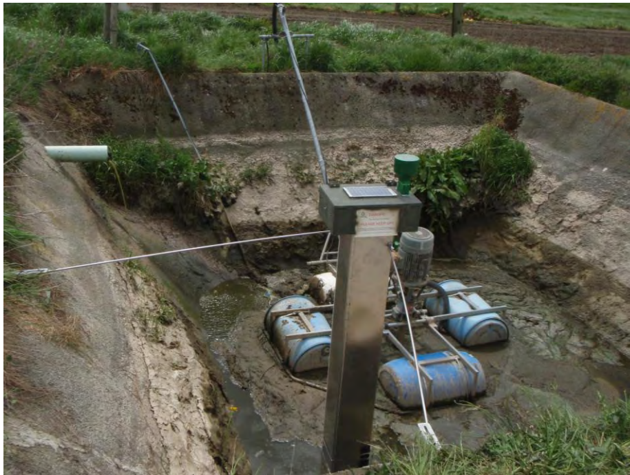
Figure 79 - Float based sensor, Wreys Bush.
