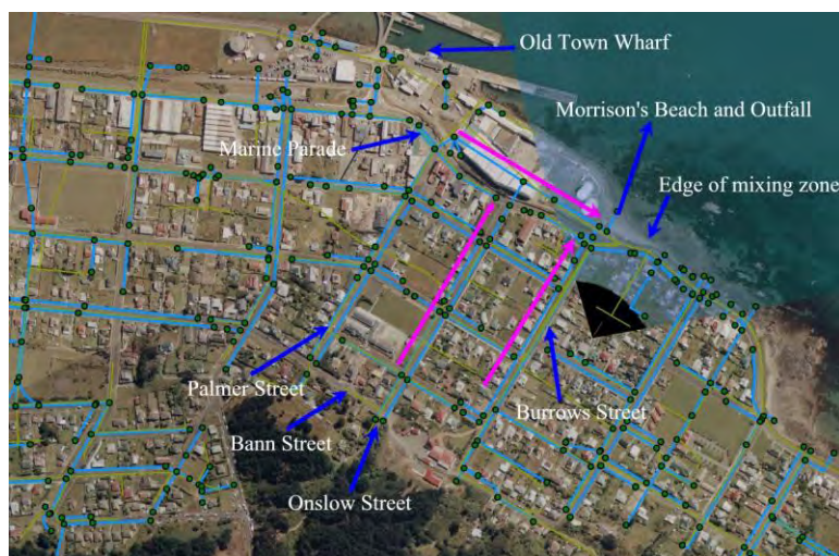
Figure 74 - Bluff Township layout and reticulated foul sewers (green lines), stormwater line (blue lines), manholes (green circles) and flow paths (pink lines).
