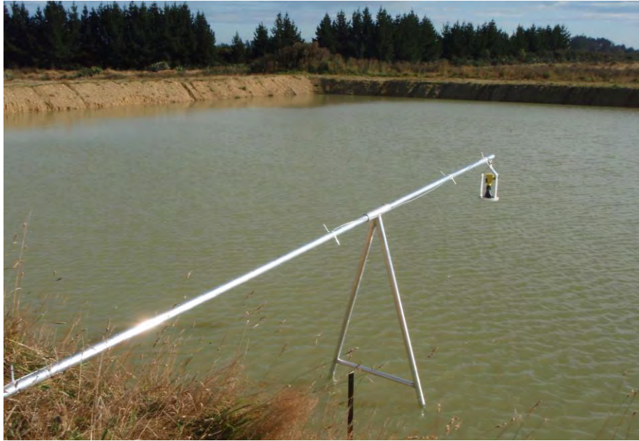
Figure 78 - Radar sensor, Waituna.
