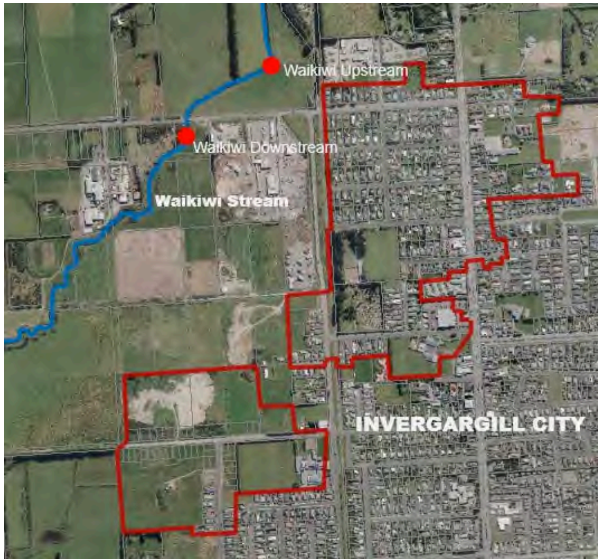
Figure 15 Map outline of sampling sites and locations along the Waikiwi Stream, Invercargill City (blue line). The Waikiwi sub-catchment of the ICC stormwater network is outlined in red. The direction of river flow is from the top to the bottom of the map.
