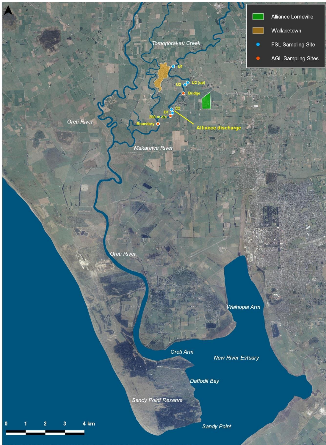
Figure 5: Aerial map of lower Makarewa River, Oreti River and the New River Estuary showing the locations of the discharge and sampling sites.
