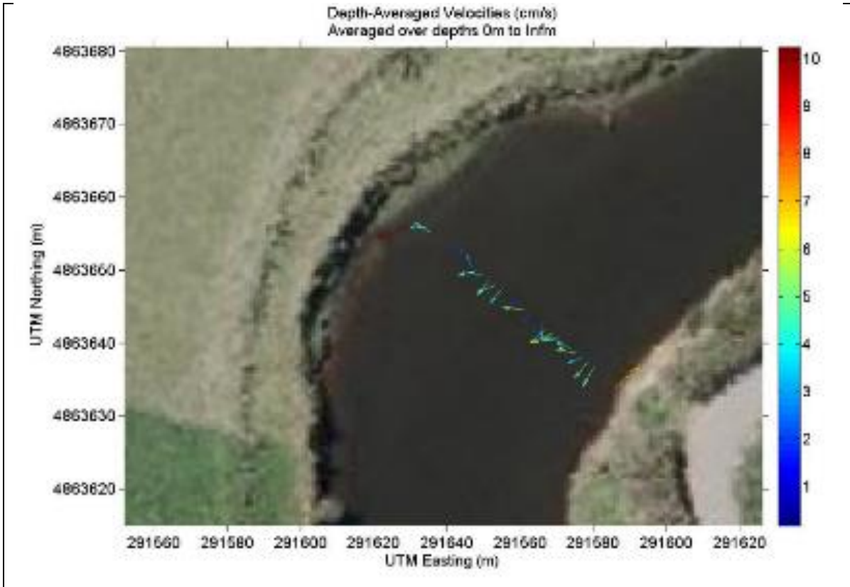
Figure 13: Depth averaged velocities at 200 m upstream cross section at high tide.
