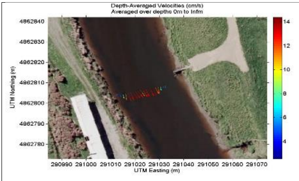
Figure 11: Depth averaged velocities at 1,200 m downstream cross section at low tide.
