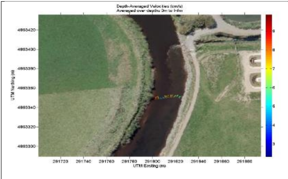
Figure 17: Depth averaged velocities at 50 m downstream cross section at high tide.
