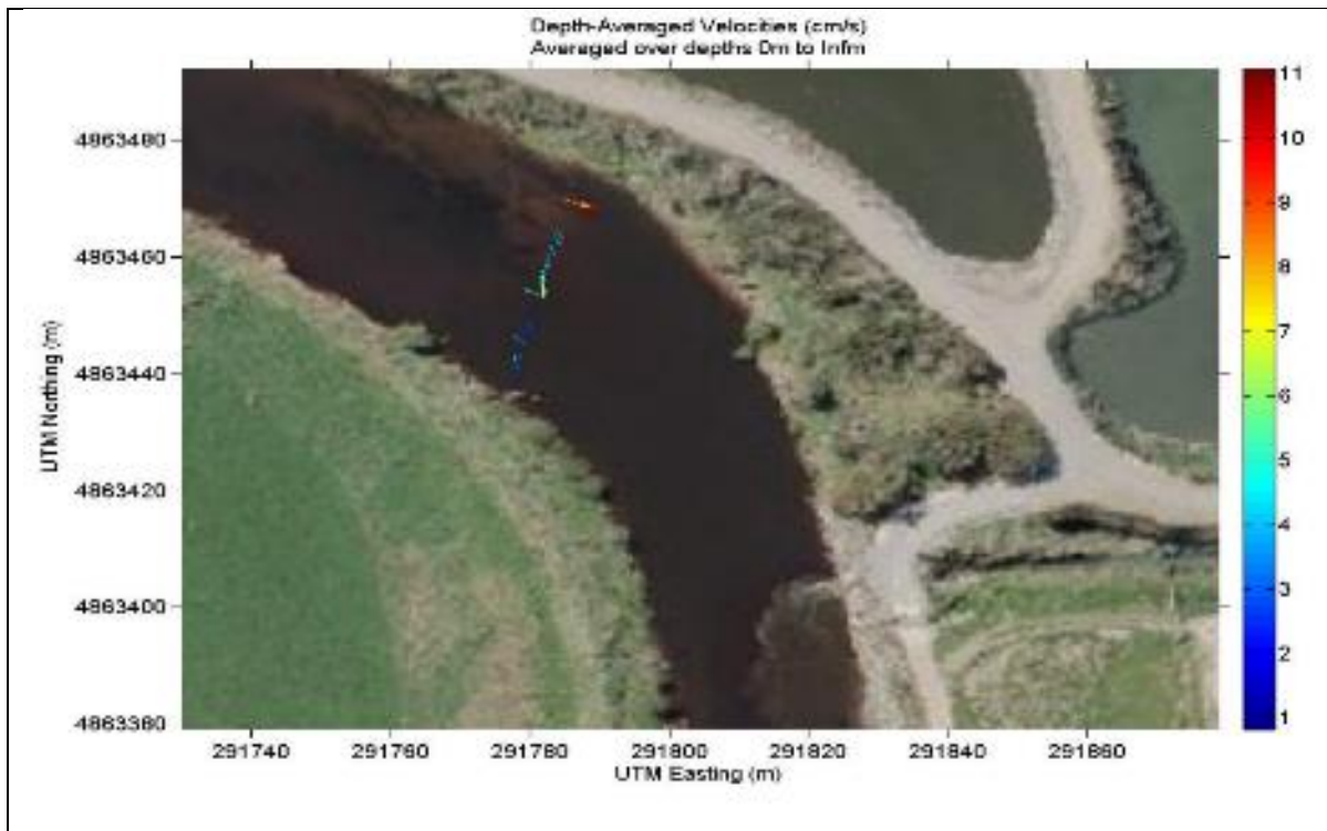
Figure 15: Depth averaged velocities at 50 m upstream cross section at high tide.
