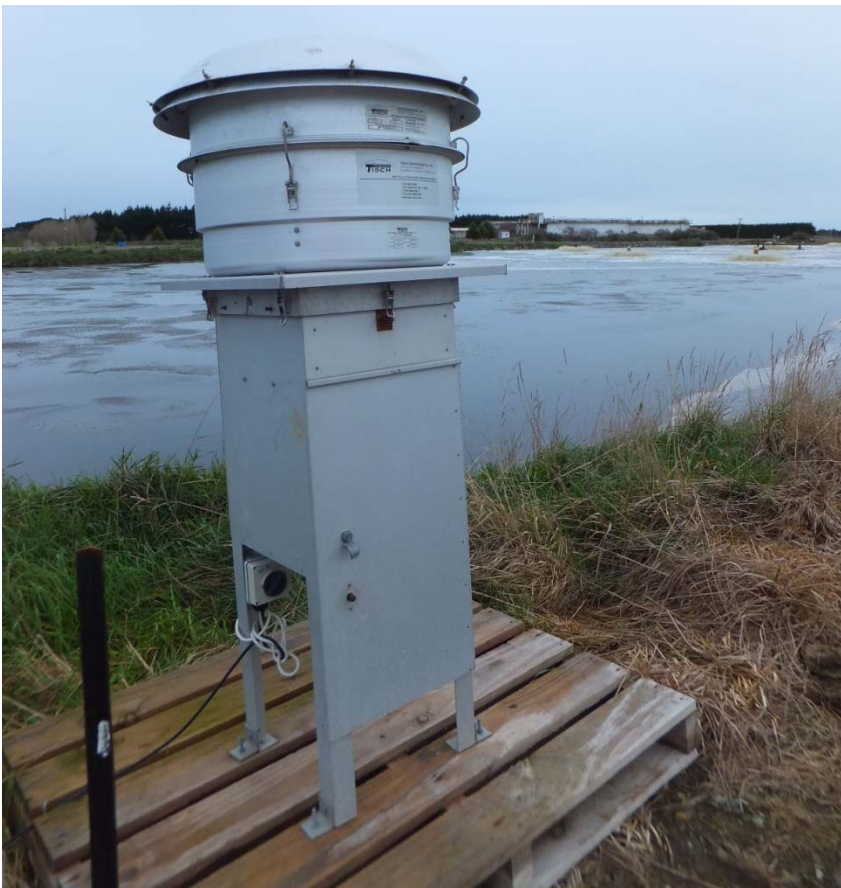
Figure 3: Photograph of the high volume sampler installed at the Alliance Lorneville 2013 monitoring site.
