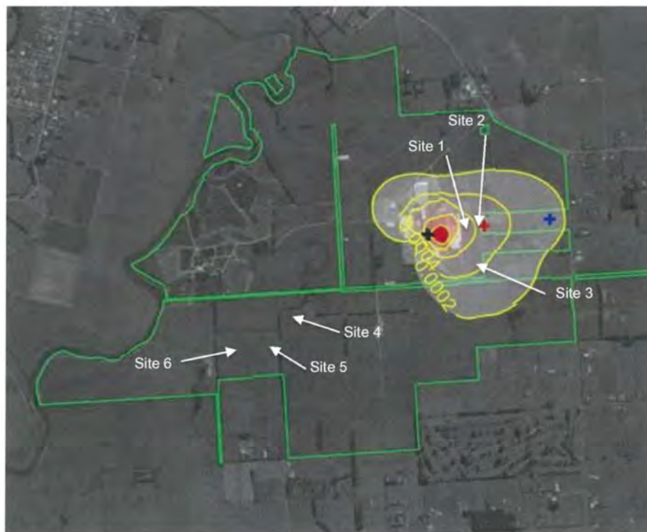
Figure 2.1: Map of relative boiler air discharge concentrations and soil sampling sites. (Map of site and boiler discharges is from Golder Associates Ltd).
