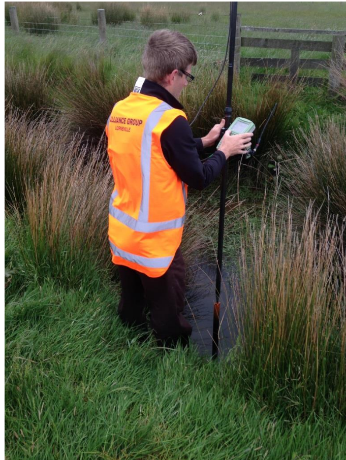
Figure 3b: Surveying the metal waratah measuring point at site S1.
