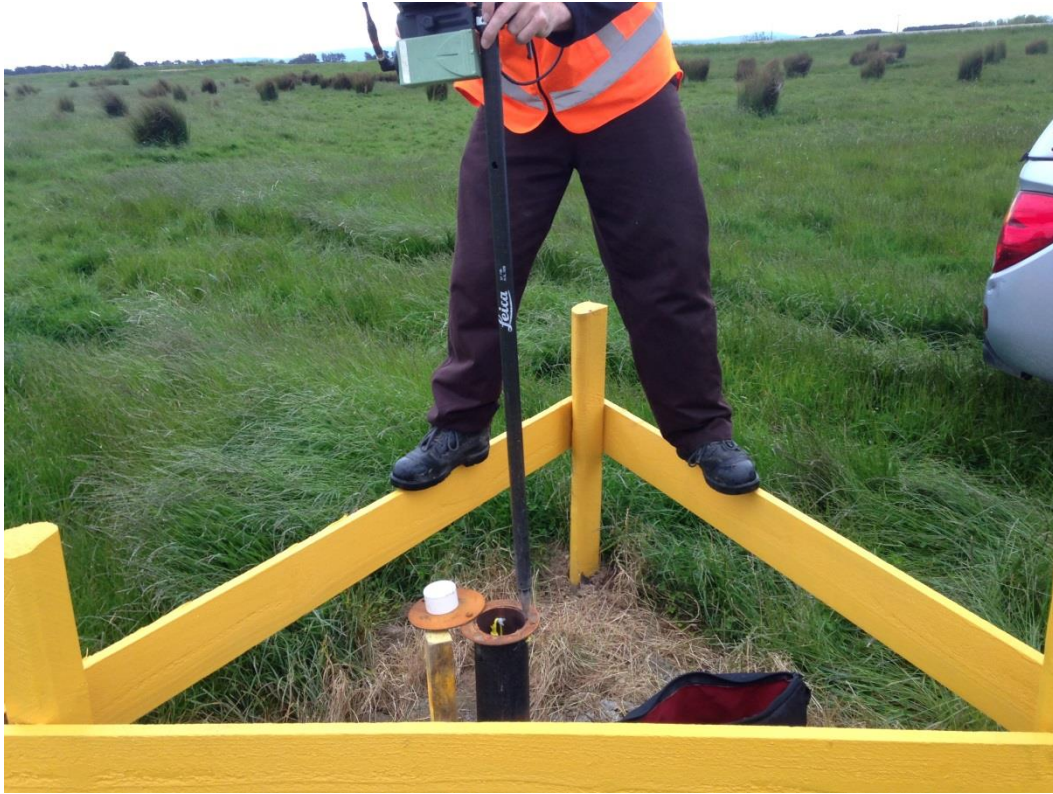
Figure 3a: Surveying the rim of the metal casing of BHD.
