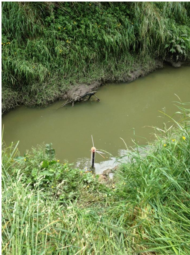
Figure 6b: Water level measuring point at site BD3 in the Boiler Ditch.
