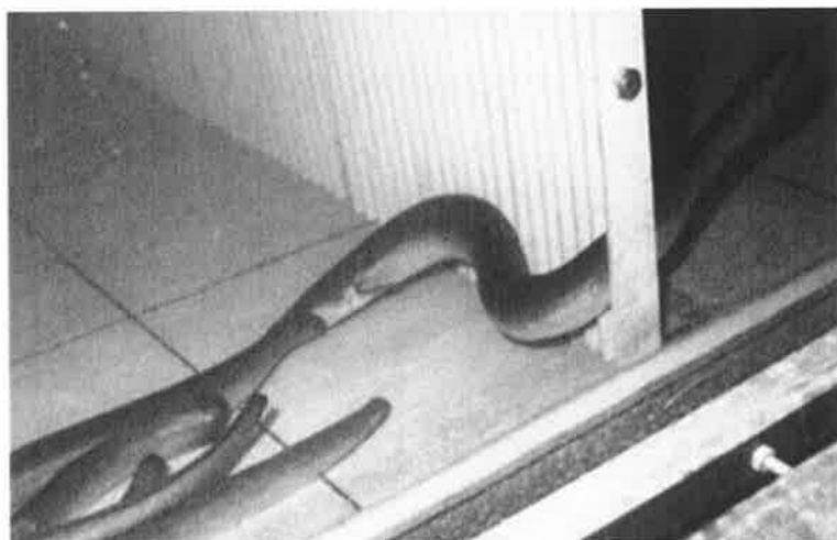
Figure 5-1: European eels (length 0.7 to 0.9 m) passing through an intake screen grate with 20 mm spacing and approach velocity of 0.9 to 1.0 m/s. (Photo - U. Dumont pers. comm.).
