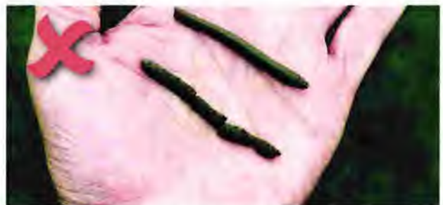
The soil makes a 'worm' when rolled, sticks to your thumb when rolled or free water appears when squeezed.
