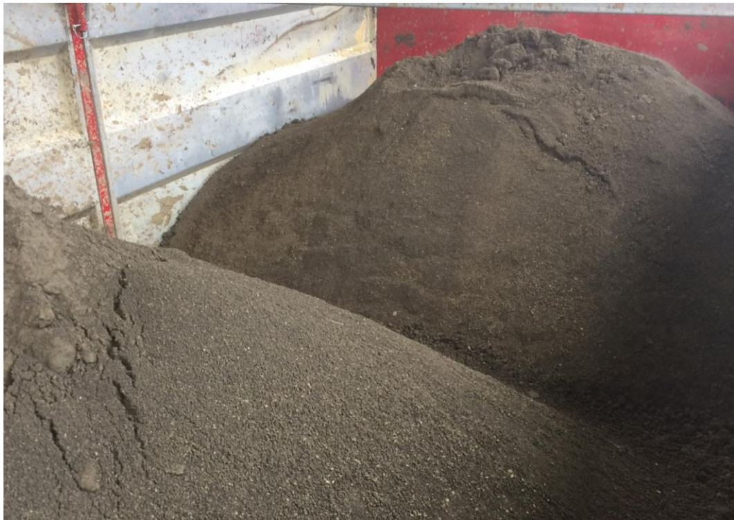
Figure 9: Final dried DAF solids ready to be taken off-site for composting.
