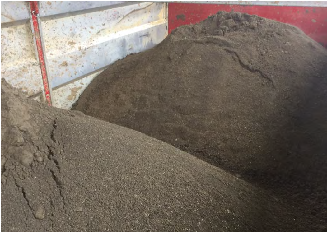
Figure 5: Final dried DAF solids ready to be taken offsite for composting.
